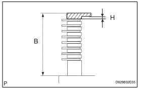
(b) Using vernier calipers, measure the level difference (length A) between the upper surface of the 1st and reverse brake piston and the hitting surface of the No. 4 brake flange at both ends across a diameter, and calculate the average. NOTICE:
