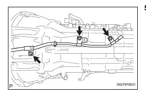
(b) Install the transmission case adapter sub-assembly with the 8 bolts.
