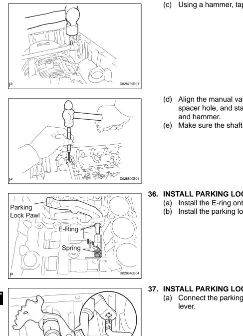
(c) Using a hammer, tap in a new spring pin.
