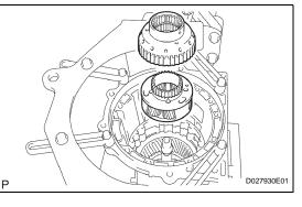
(c) Install the front planetary gear assembly and 1-way clutch inner race into the case.
